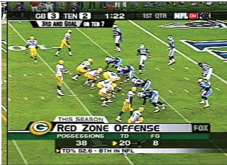
Figure 6.46 Below and on the opposite page is CBS's version of the Fox box in the upper left corner, generated by SGI O2, lower banner Chyron iNFiNITI, and first-and-ten PVI. The score in the upper right is a linear key that is usually provided by a Digital PC Codi. In most cases today, the stats in the lower banner are automatically provided by a third-party statistic vendor via a database, which the CG automatically loads into a template. The right shows FOX's latest version of the Fox box, which now is more of a ribbon than a box.
