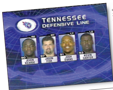
Figure 6.44 Lineup out of SGI Q2 based on a template that looks to a database for objects to comprise the display. Those objects include the moving background, and player positions, names and pictures. This graphic is only composited into a complete graphic when it is called up by the graphics operator.
