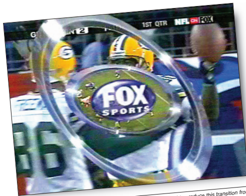
Figure 6.47 Graphics and the production switcher work in concert to produce this transition from game to replay. Two channels of GVG Profile video server is used to produce the ring's key signal and video fill. At the same time, the production switcher is performing a circle wipe in step with the moving graphic.
